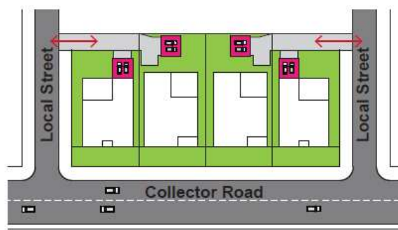
Figure 10: Options to control access to collector streets
