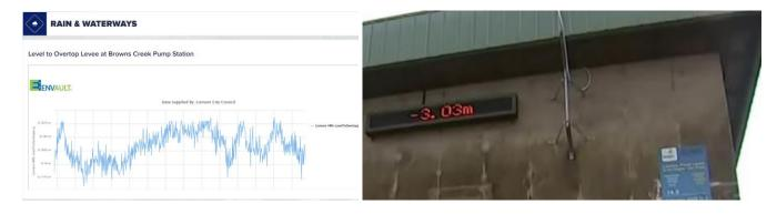
The Disaster Dashboard display will mirror the on-site digital readout at the Pump Station, showing the local gauge reading at Browns Creek (not the Wilsons River at the Lismore mAHD gauge).
