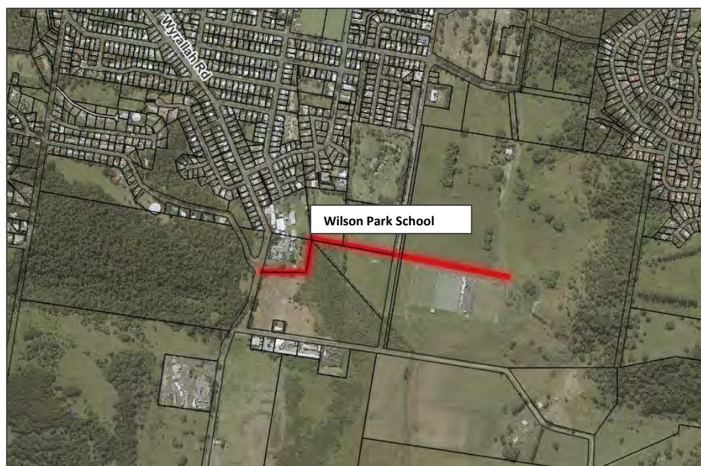
Figure 3: Option 3 Levee Alignment
