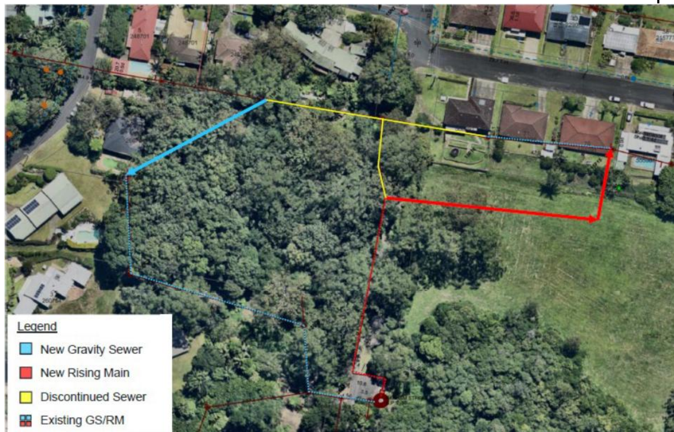
Figure 2: Proposed Sewer Re-alignment
